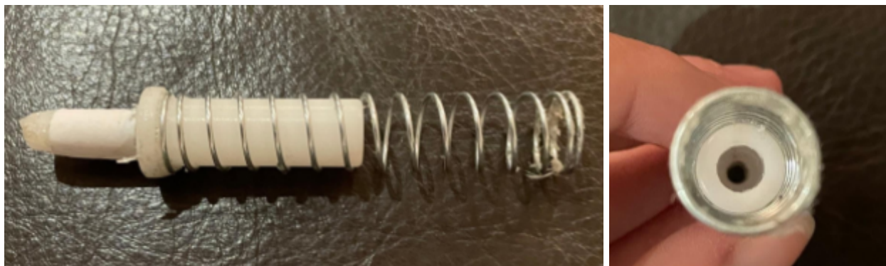
Figure 2: Spring and spring holder (left). End of the hollow spring holder (right).
